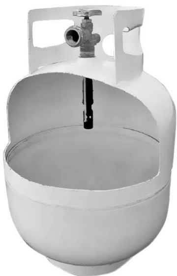
Figure 1 Appliance Cylinder VAPOR SERVICE
